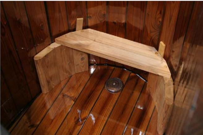
Place the first seat, included calibration pieces help to place the seat properly. Check that the seat is even towards the base.
