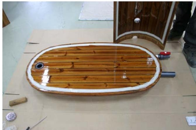
Put the pipe on the underside of the base and screw the valve in place with the included wooden tool.
