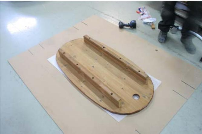
Assemble support legs, there are pre-drilled holes for fastening the legs already marked on the base.
