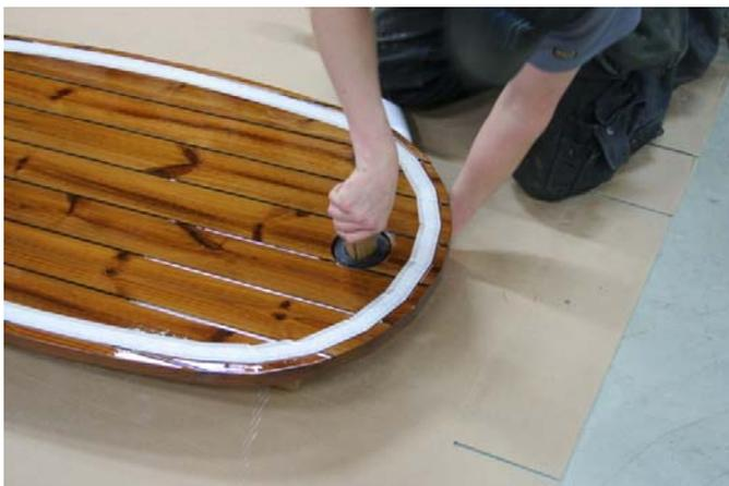
Use the included tool in wood to screw the drainage valve in place.
