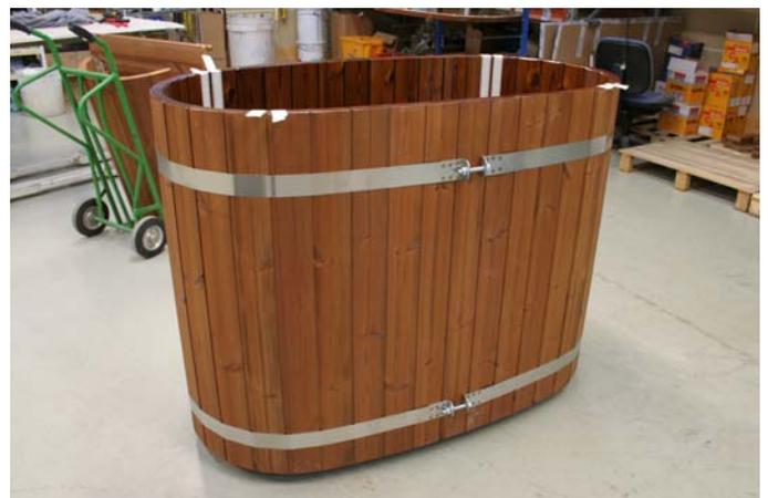
Place the stainless steel bands on the nails and tighten the bolts until the space between them is around 40 mm. While the bolt is tightened, walk around the tub and tap the sides with a rubber mallet in order to adjust the modules so that the bottom seam is the same width all around.
