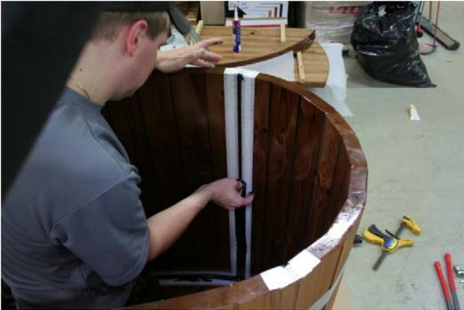
Smear out the sealant in the side module seams with a filler spreader.
