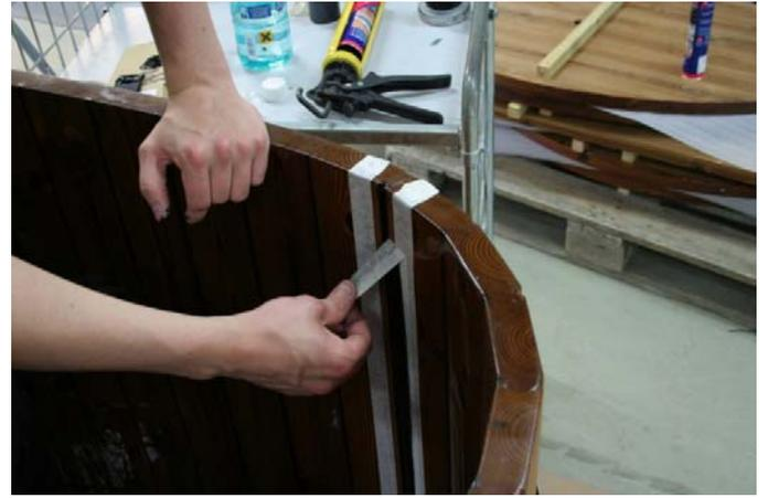
Remove the masking tape and let the seams dry for at least 12 hours..
