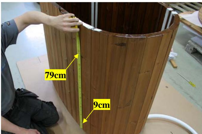
Attach support nails for the stainless steel bands in every corner of the hot tub. Measure 9 and 79 cm from the bottom of the side module.
