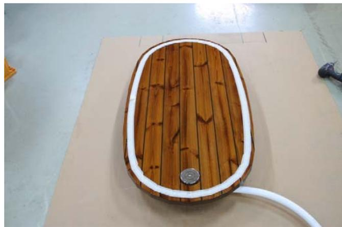
Screw the valve cover in place.
