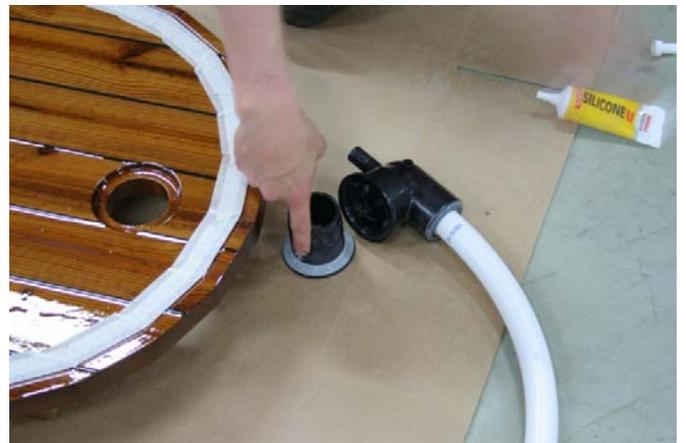
Smear out the silicone on the threads with a finger.
