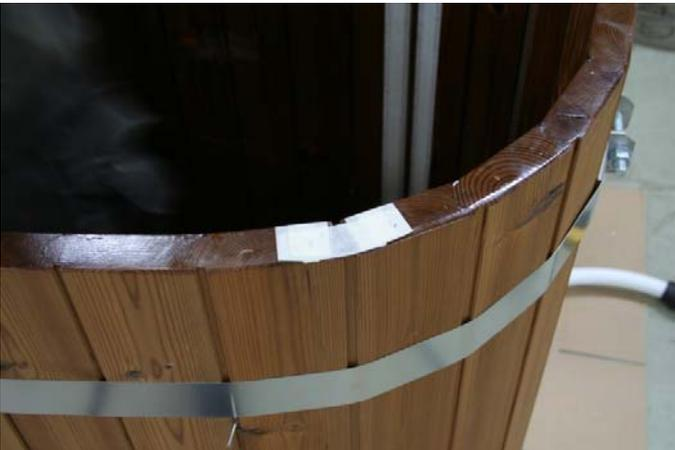
Put a bit of extra masking tape on the top as the picture shows, to make a prettier seam.
